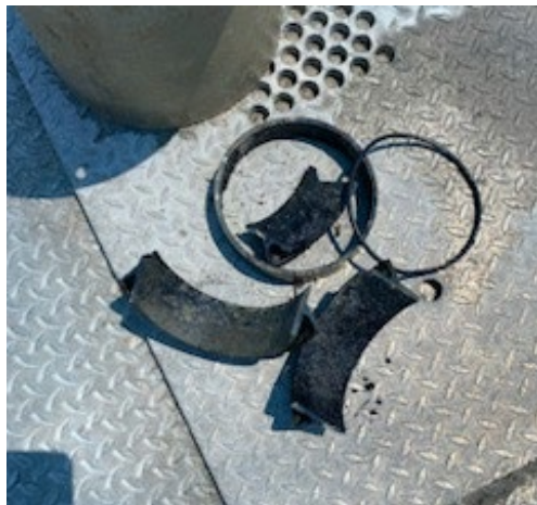
Photo: Broken cascade ring (left), sand filter wash zone assembly (right)
